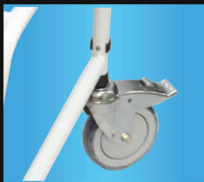
Quick release black clips can be removed and placed in adjacent holes to change caster height
